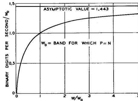
Fig. 7. Channel capacity as a function of bandwidth.
